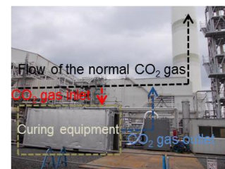
Curing equipment of CO 2 -SUICOM
